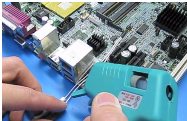
Figure 20 Using low-temperature hot glue to secure a probe head
